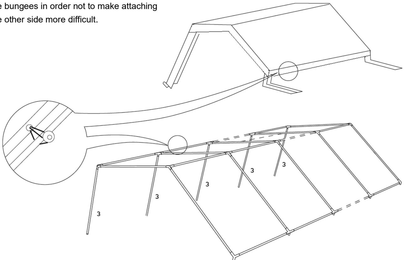
**3.** Attach the legs on the other side. Make sure, that the leg pipes are in vertical position, to avoid overtention on the endwalls. Attach legcover to the legs with hooks ..
