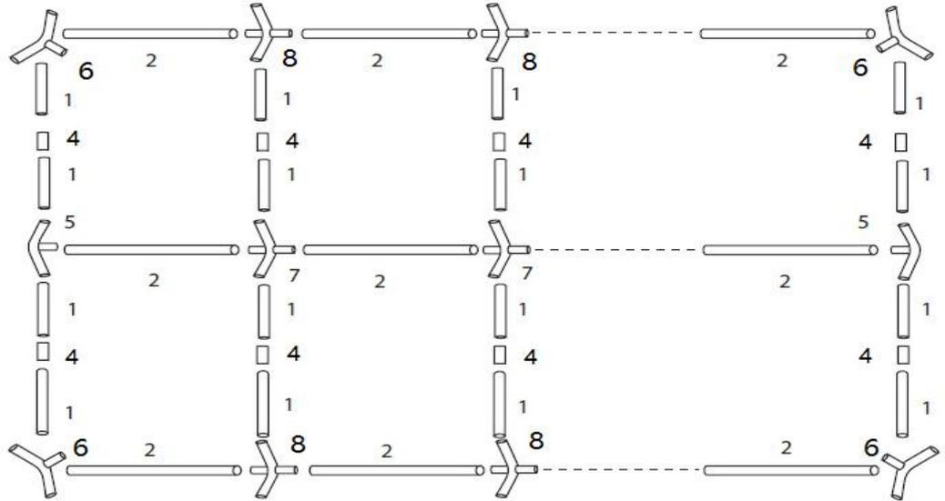
2. Lift one side of the tent frame and attach the legs (3).
